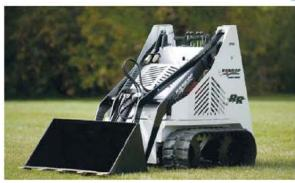
small places. Machines are driver-friendly, with an unobstructed view of all working conditions. The 34-inch or 40-inch narrow track base of the RAMROD Estate Series makes it easy for operators to access tight work areas that larger loaders are incapable of reaching. These compact machines are easily transported on trailers or pick-up trucks and are ideal for homeowners, acreages, barnyard use or light-utility and construction applications.
