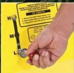
The first reciprocating aerator on the market that allows the operator to determine a comfortable operating speed from approximately 2.5-3 MPH. This speed adjustment feature allows variation for landscape complexity, lawn size, operator safety and maximum productivity.
