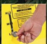
The first reciprocating aerator on the market that allows the operator to determine a comfortable operating speed from approximately 2.5-3 MPH. This speed adjustment feature allows variation for landscape complexity, lawn size, operator safety and maximum productivity.
