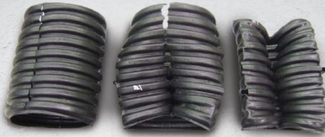
Standard pipe ASTM Crush Test Samples
