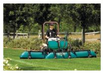
independent suspension and dolly wheels follow ground contours for precise and even spray application. Each spray chamber features four spray nozzles, which provide uniform coverage by applying finer spray droplets that coat vegetation instead of dousing it. Combined with True ZeroTurn maneuverability to avoid wasted motion, the result is up to 5.5 acres per tank — with fewer chemicals, faster application times and faster drying times. *GrasshopperMower.com/sprayer*
