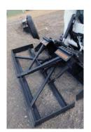
crumbler beam knocks tough earth into manageable dirt, enabling the V3 FlexPlane to tackle terrain. Sizes include 72-, 78-, 84-, 89- and 96in. models. *Grouser.com*
