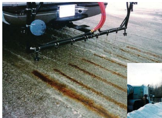
◀ A spray truck disperses a sugar beet-based deicer on the highway.
