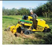
The unit features the optional AutoSweep monitoring system from Vermeer, and a combination belt and gearbox direct drive system offers an efficient transfer of horsepower from the engine to the cutter wheel. An operator presence system monitors the operator's touch and maintains cutter wheel engagement. When the operator's hands leave the control levers, an automatic disengage and braking sequence will stop the cutter wheel in less than nine seconds. *Vermeer.com*
