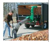
cal intake hose with user-friendly handles and hose connection for improved hose management and maneuverability. The unit can be skid-mounted as standard; options include a tailgate mount or swing-away truck hitch. *BillyGoat.com*
