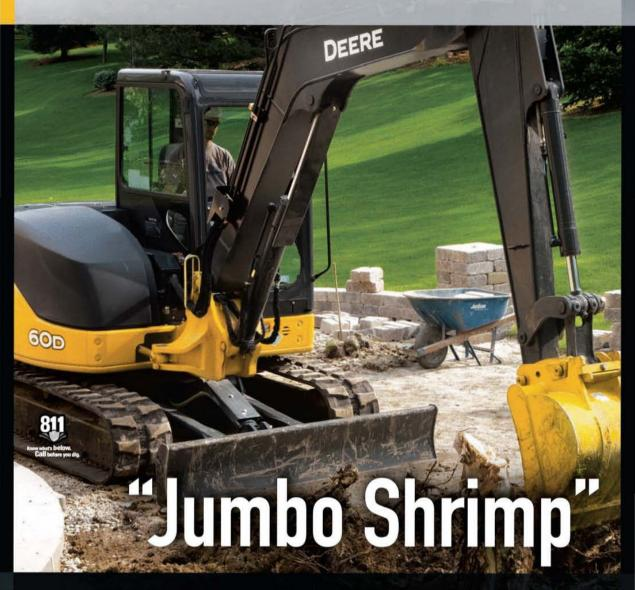
As compacts go, it's a freak of nature. With its standard swing boom, reduced tail swing, backfill blade, and rubber tracks the new 60D Excavator works in tight spots like our other compacts. But this true 6-metric-ton machine boasts big-machine features, too, such as a standard cab, pattern changer, more than 7,000 pounds of lift capacity, and over 13 feet of digging depth. See your dealer or call 1-800-503-3373, because you shouldn't have to choose between big and small.
