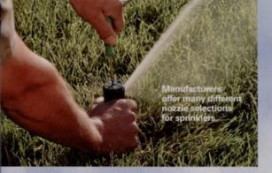
much pressure breaks up the spray pattern, causing small droplets (misting) that reduces the radius of the spray pattern. Too little pressure, and the drops of water are too large, and the area immediately surrounding a sprinkler gets too little water.
