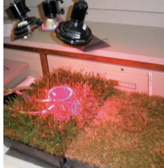
An infrared gas analyzer tests the carbon sequestration capabilities of tall fescue (left) and bermudagrass (right) at Bayer's Clayton (NC) Development & Training Center.
