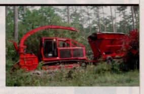
ing and powering an agricultural dump wagon to collect material. Material is chipped using Fecon Bull Hog chipper knives or carbide tools, then augured to a material processing fan and blown into a collection unit. It can discharge from the rear or the side, enabling a variety of collection units.
