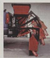
power down pressure scrapes the surface cleaner, reducing the amount of deicer material needed for ice management. For more information contact 888/766-6267 / www.snowmanplows.com / circle no. 253
