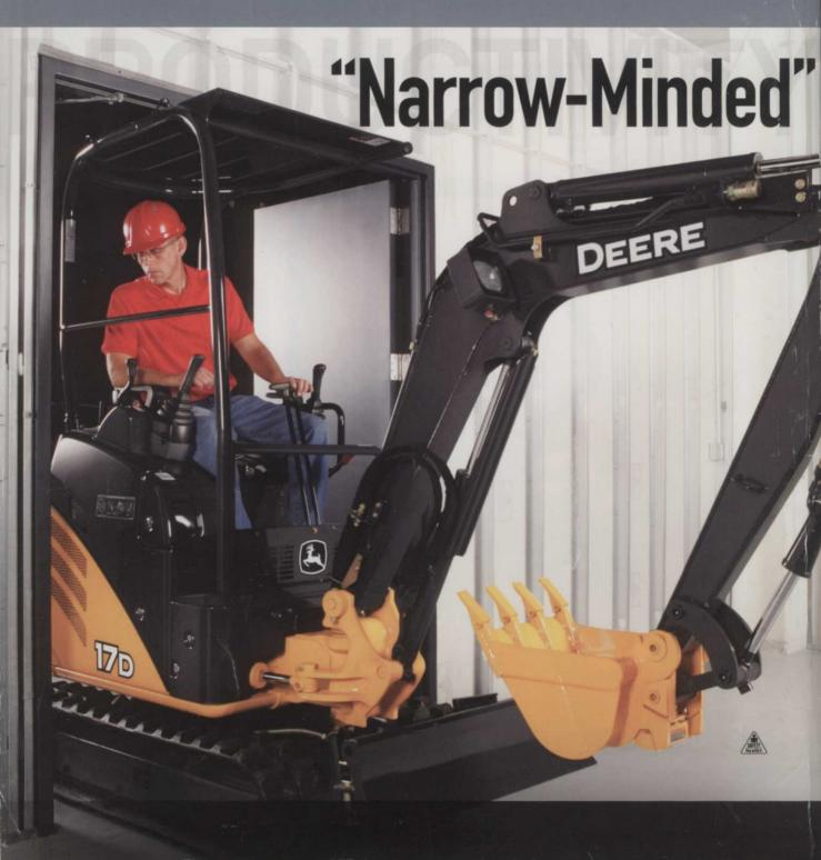
The new compact 17D has a one-track mind for maneuvering in conservative spaces. Its hydraulically retractable tracks and folding backfill blade help get you in and out of tight quarters with a minimum width of just 39 inches. Then, when you're ready to work, the tracks expand to over 50 inches for stability. Talk to your dealer or call 1-800-503-3373 to find out how a narrow-minded 17D Compact Excavator can expand your possibilities.
