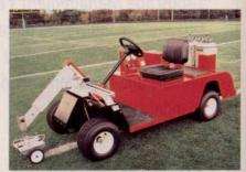
vides straight lines. Two 12-gal. steel tanks are controlled by a switch near the seat. A hydraulic spray arm sprays sharp, straight lines in front, or can be moved to the side for crisp circles. For more information contact Pioneer Manufacturing at 800/877-1511 or www.pioneermfg.com / circle no. 255
