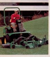
72-in. 7-Iron V-Flex mower deck answers landscapers' demand for a rotary mowing deck that provides superior performance on flat and uneven terrain. A rear wheel kit offers 1- to 5-in. heights, while a
