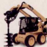
4 High Lift Models Skid Steer Loaders Operating Capacity: 1,750 - 2,500 lb 30+ Work Tool Types*
