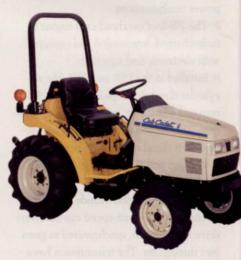
Two- or four-wheel-drive operation keeps tractors from turfing in two-wheel drive and provides maximum traction to operate with four-wheel drive in rough terrain
