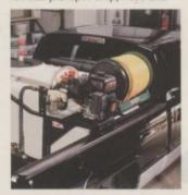
engine are accessed from curbside of truck. Powered by Kawasaki 5.5-hp FE-series engine and Hypro 403 series 3-piston diaphragm pump. Hannay electric hose reel has 300 ft. of 1/2-in. 800 psi ure-thane inner core hose.
