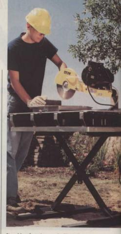
Stow Manufacturing says its TP-10 tile/paver saw is capable of ripping a 24-in. tile in a single pass or cutting an 18-in. tile diagonally. Powered by a totally enclosed, non-vented 1.5-hp electric motor, its blades range from 7 to 10 in. A 10-in. blade is standard, and additional blades and profiling wheels are also available. For more information contact BOMAG Light Equipment Division at 800/235-0008 or www.stowmfg.com or circle no. 280
