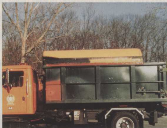
The top of a schoolbus salvaged from a junkyard became a portable roof for Phillips' dump body.
