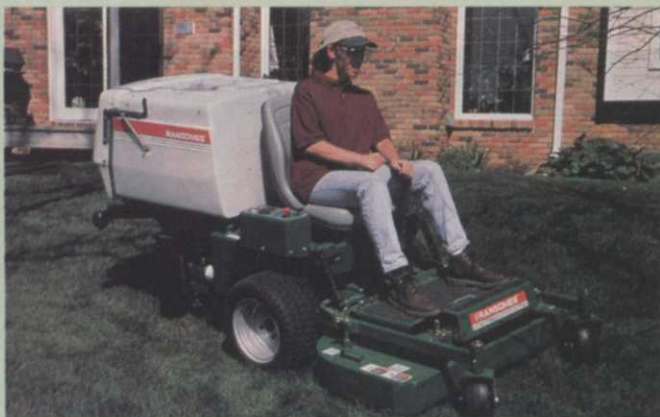
The Bob-Cat ZT 100 features independent power and control to each wheel for enhanced maneuverability.
