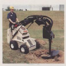
crews do more work faster, and with fewer personnel. A 25-hp Kohler engine generates a hydraulic flow rate of 13.4 gpm. Full power is delivered to wheels and tools at same time. Oil cooler is standard. Quick-change feature allows attachment changes in less than one minute. Over 30 attachments are available, including trencher, tiller and box rake.
