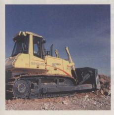
cycles by automatically shifting from forward to 2<sup>nd</sup> reverse when reverse is selected. Fingertip steering and transmission controls require little operator effort. Wide-opening service panels, diagnostic test-port panel and other features reduce maintenance time.
