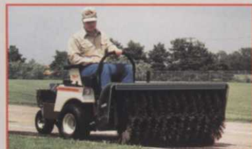
PTO-driven 48- and 60-inch fixed angle rotary brooms handle dirt, debris and clean up to eight inches of snow. 60-inch bidirectional broom available.
