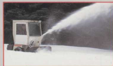
PTO-driven 48- and 60-inch snowthrowers throw snow up to 20 feet away. Winter enclosure for all snow removal attachments provides protection from wind and snow.
