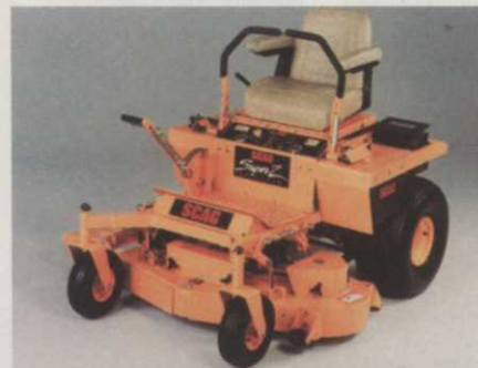
Scag Super Z with electric blade engagement
