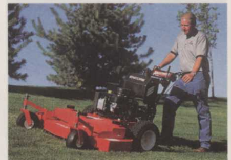
Encore Premier has removable fuel tank
