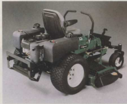
Lesco Viper features articulating front axle
