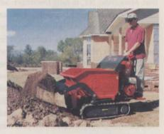
This imported unit has a retractable track system that reduces its width down to only 30 in., small enough to fit through gates. Less weight and minimum ground pressure dispersed evenly over the track system means the unit is less likely to damage lawns or other prepared surfaces.
