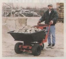
Honda's 5- or 5.5-hp engines move the unit at a comfortable walking speed. A 360° rear swivel wheel gives the Haulzall more maneuverability. Attachments include a flat bed, dolly, trailer hitch, snow blade and hydraulic lift-dump cylinder.
