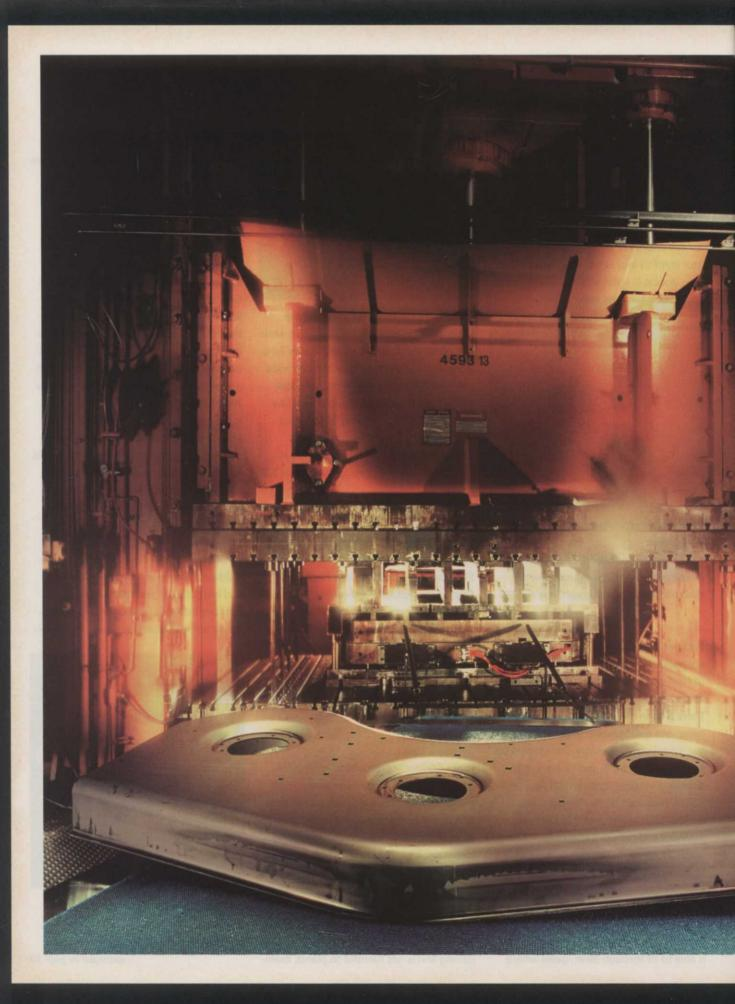
JEON Its inspiration was the passion to build the best. Four years and four million pounds of pressure later, it's finally ready. Introducing the 7-Iron™ mower deck from John Deere. Stamped from a single sheet of incredibly thick 7-gauge (.177 inch) steel, in the industry's largest press, its perfectly smooth and impossibly strong shell (shown to the left) has no welds to break, or irregular
