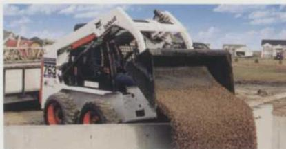
The long-wheelbase 763 loader is a smooth-riding machine with plenty of traction and breakout force for excavating and handling large loads.
