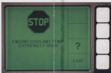
For example, this screen appears if the engine coolant temperature is excessively high. Push the "question mark" icon for further information.
