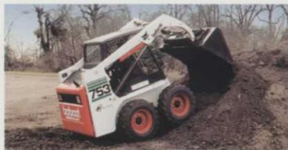
The 753's large tilt cylinder and rollback power mean improved digging and loading capability, and its tight turning radius lets you handle big jobs in small areas.
