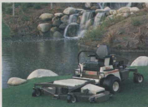
28 hp 928D 2 with heavy-duty 72-inch deck.
