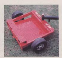
The sulky can be disconnected quickly with one pin and the adjustable hitch allows it to be attached to almost any brand of equipment. For more information contact Jack Ball at 323/258-4135, fax 323/258-3376 or Circle No. 272
