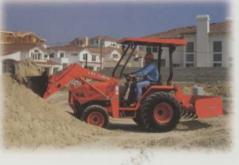
and L35 have a convenient single-lever/ dual function control with an increased lifting capacity. The backhoe is a cinch to quick-attach while the rear PTO and 3-point hitch maximize
