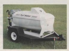
mount on a flatbed truck along with an auxiliary water tank or will fit into the back of a pickup. It is also available mounted on a trailer with a 5,000-lb. axle, electric brakes and heavy duty tires. The unit can be removed from the trailer if desired.
