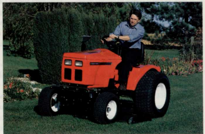
Power King tractors are shaft driven. The UT 622HV is powered by a 22-hp Kohler engine.
