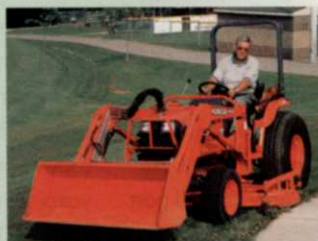
Kubota's 20-hp (at the PTO), 4WD tractor features single-pedal control
