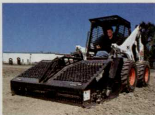
Landscape Rake grades, levels and picks up debris.
