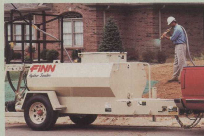
Finn Corporation's T30 HydroSeeder is an entry-level machine for establishing new lawns. It has a 300-gallon capacity.
