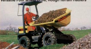
The Thwaites 5000H Powerswivel Dumper features a 1.8 cubic yard bucket that swivels a full 180 degrees to dump left, right, or anywhere in between. Its small size, 4WD, and hydrostatic transmission make it perfect for shuttling soil, concrete, or other materials in confined spaces or rough terrain applications. Larger models available with 2.3, 4, and 4.7 cubic yard capacities.
