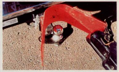
damage to the bumper and license plate and is easy to assemble and remove. The two-part system consists of the base plate, installed under the hitch ball, and the V-guide which fits into the slots of the base plate.
