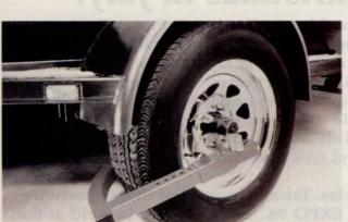
Keeper is adjustable to fit wheels up to 15" and can be used on almost any type of trailer.
