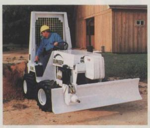
positions enable trenching in any type of terrain. The 4500-pound unit is equipped with hydrostatic drive.
