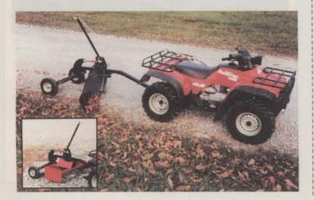
pull lever to raise the unit while turning or dumping and a clevis-type hitch.
