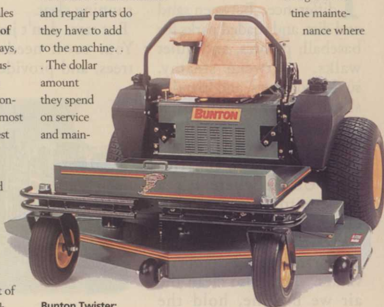
Bunton Twister: available in 48- 52- and 61-inch cutting widths.
