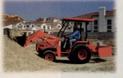
and L35 have a convenient single-lever/ dual function control with an increased lifting capacity. The backhoe is a cinch to quick-attach while the rear PTO and 3-point hitch maximize
