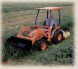
While the L35's new generation Glide Shift Transmission operates all eight speeds and reverse without clutching.
