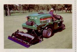
ways or sports fields, the unit's subsurface shattering process also helps reduce soil compaction, increase microbial activity and improve percolation.
