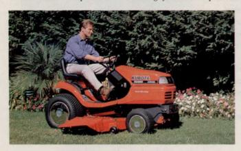
control without loss of horsepower while turning. Also standard on the TG series is Kubota's Cushion Ride suspension system, two spring-loaded shocks connected to the flat operator's deck.
