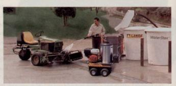
of three tanks, a grass clipping removal assembly, and automated pumps for controlling the use of BioStax GC, the proprietary solution of microbes that breaks waste like oil, grease, hydrocarbons, and grass clippings into harmless substances consisting mainly of carbon dioxide and water. The resultant water can either be dis-
