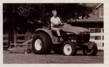
diesels, have hydrostatic power steering and are equipped with wet-disc brakes.
