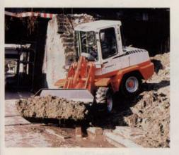
Schaeff Equipment offers joy stick control on its new SKL 823 and SKL 833 wheel loader/tool carrier models. "In addition we have added 20 percent more glass in the cab for increased operator visibility," says Gil Herr, president of HAMM, the U.S. distributor. "The machines continue to feature parallelogram linkage which keeps the bucket level with the ground, even at a maximum height."
