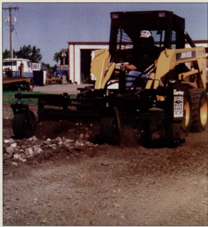
Harley power rakes level ground, pulverize the soil and remove stones and other debris. Features include twin-drive rollers, oil-bath drives, splined power shafts, hydraulic float control.
