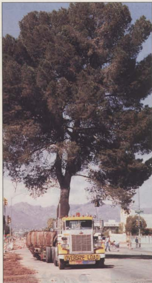
With the 'boxing' method, steel plates are fastened to the rootball for overland transport.
