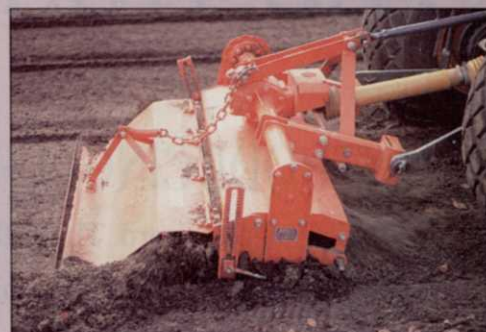
Napier roto-tilled the nursery with the tiller set at a depth of eight inches.
