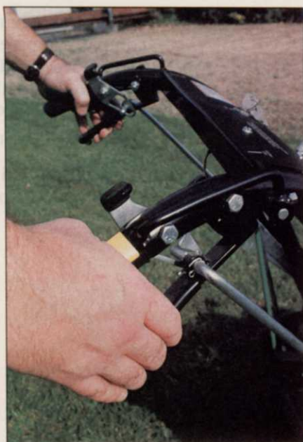
▲ An operator's hands must be at the controls for modern machines to keep operating.
