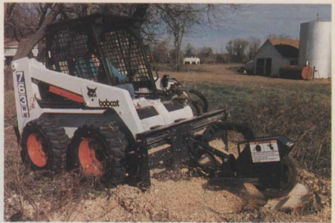
The SG50 stump grinder with the 763H Bobcat. Its 3-inch wide cutting head has 34 teeth, and cuts down 20 inches below grade.
