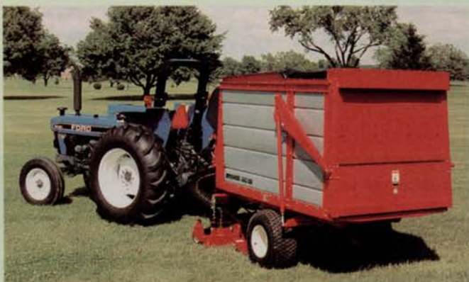
Brouwer - Vac 138 is suited for large-area collection of debris.
