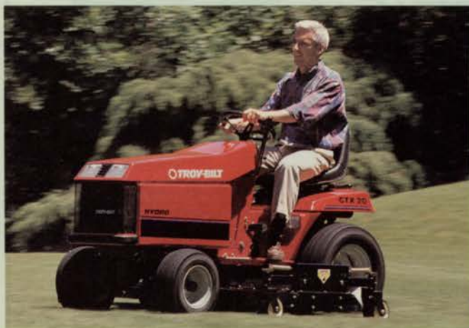
Troy-Bilt GTX with single-pedal hydrostatic drive, power steering
