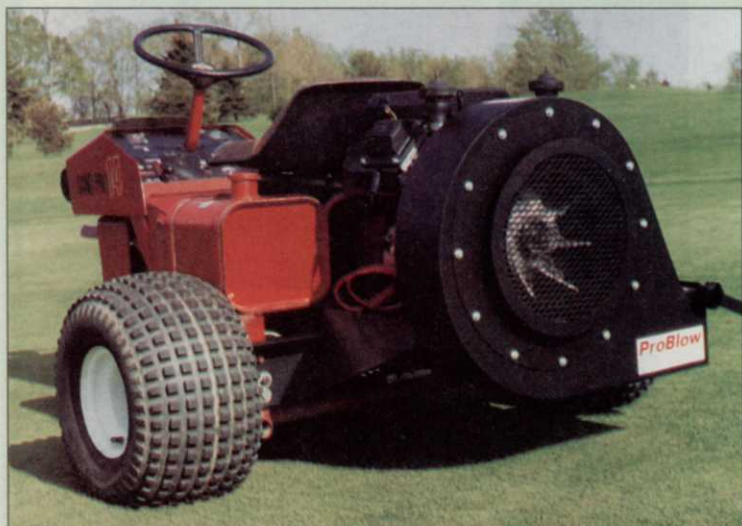
Selbro Pro-Blow mounts to Walker ZTR mower.
