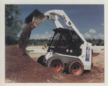
751 offers a compact footprint for a mid-size loader with a turning radius of less than six feet. The 751 has a 1,200-lb. operating capacity, using a 116-cu. in. Peugeot XUD9 diesel engine, and many standard Bobcat C-Series features, including a dependable transmission with heady duty drive chains that never need adjustments and the exclusive Bobcat Interlock Control System.
