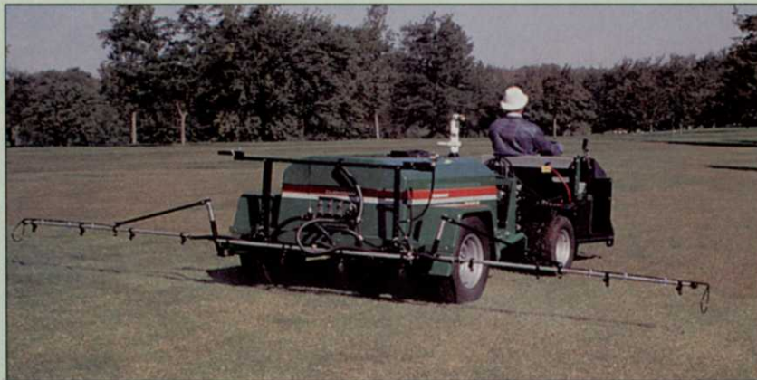
The Cushman 5th Wheel Sprayer contains six Venturi Jet agitators.
